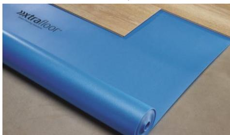
Xtrafloor™ Base & Xtrafloor™ Flex Pro, as recommended above, can smooth out small irregularities of a **maximum 5mm wide and 2mm deep**. This allows for installation over existing floor coverings, such as ceramic tiles, linoleum, compact PVC floors and wooden floorboards.
