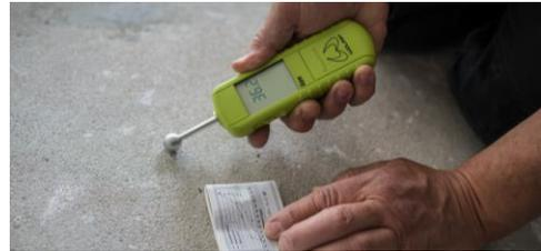
**The moisture content of the subfloor must be in accordance with local or national standards for the installation of resilient floorcoverings. If in doubt seek further advice.**
